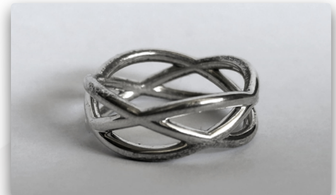
Figure 2: Lissaje ring made by loss wax casting method.
