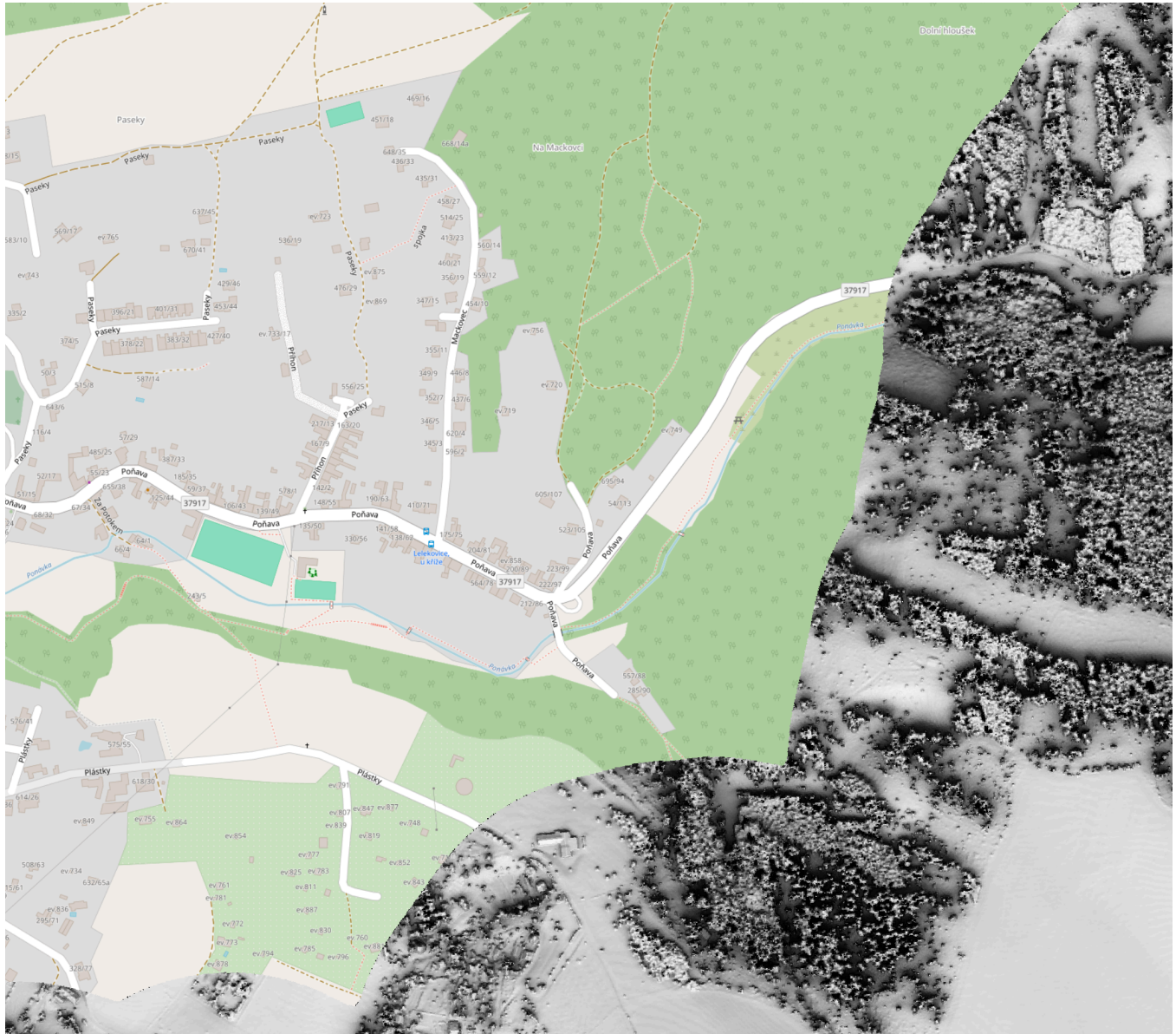
Figure 2.1: Solar Irradiance dataset of Brno (in grayscale) on top of OpenStreetMap layer (available under the Open Database License), screenshot from QGIS
