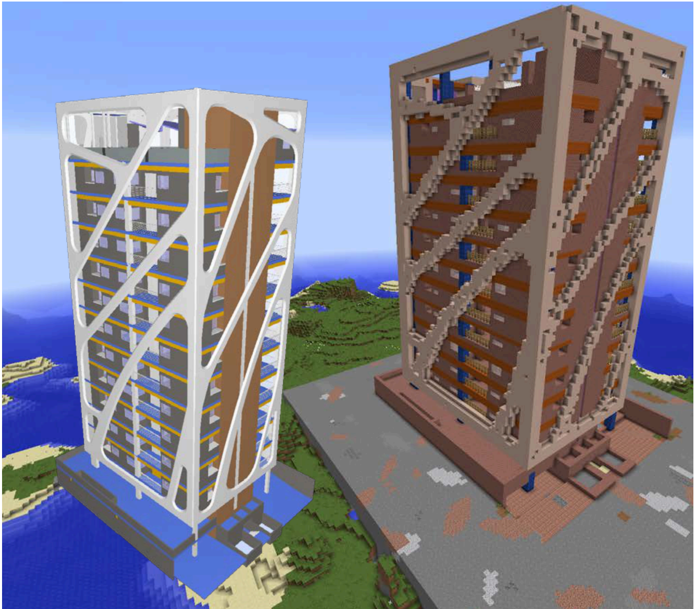
Figure 5.2: Model of a building from the ArcGIS CityEngine (left) and the model voxelized by FME (right), adapted from [11]
