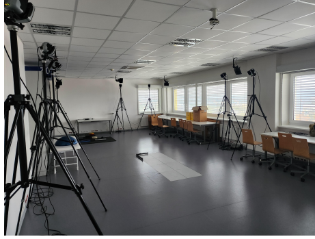
(a) Sports laboratory at FEKT BUT with Qualisys motion capture system.
