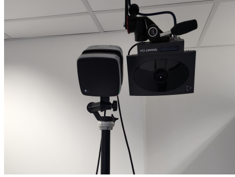
(b) Arqus camera (on the left), connected to next ones in a chain using RJ-45 connector.
