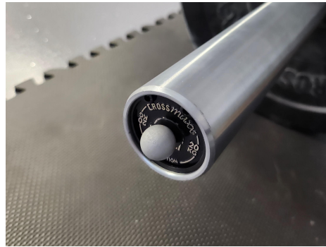
(d) Passive reflexive marker placed on the very end of a barbell.
