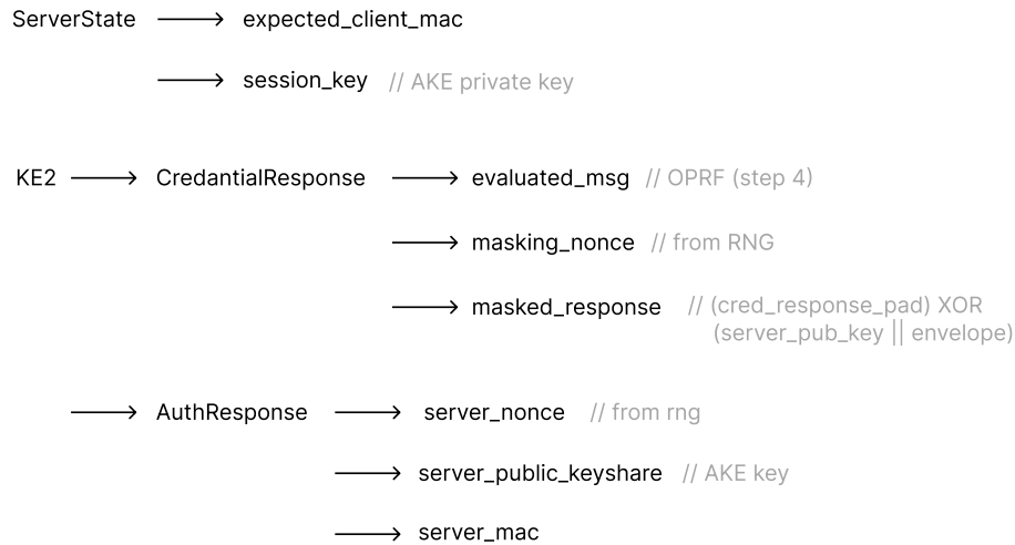
Figure 3.4: Second AKE Message Generation: Server-Side Flowchart.
