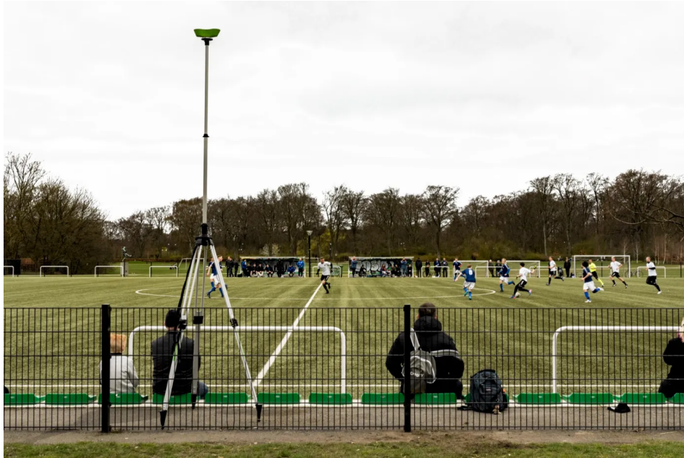
Figure 2.2: Veo Cam 2 [2] Mounted on a Tall Tripod at the Center Line of a Soccer Pitch
