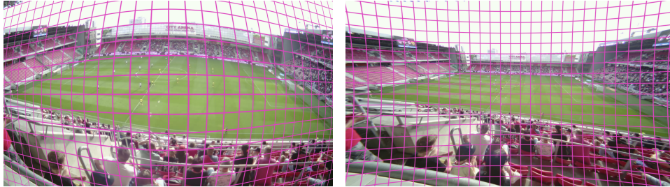
Figure 6.1: Example of barrel (left) and pincushion (right) distortion with annotated grid lines.
