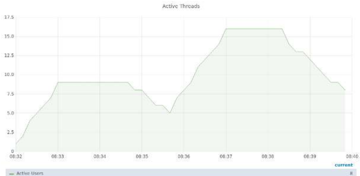
Figure 6: Thread count during performance test (source: Author)
