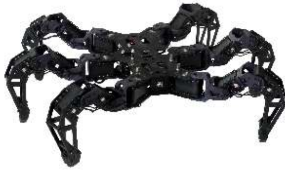
Figure 25: Hexapod walking robot Phantom X Mark II utilized in the exploration scenarios.
