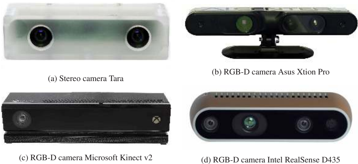
Figure 26: Sensors considered for vision-based localization.
