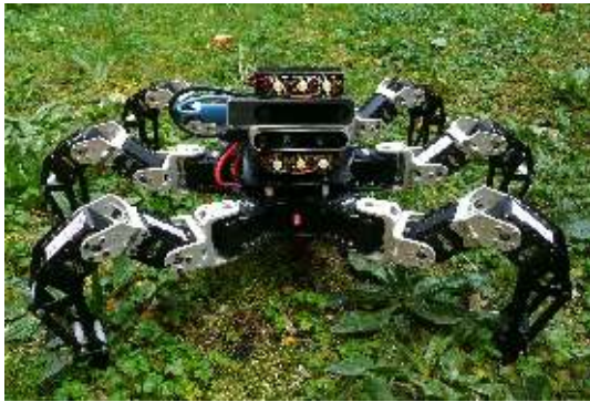
(a) Hexapod walking robot with developed sensor rig for autonomous exploration
