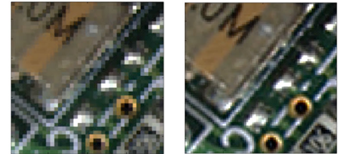
Figure 2: Input image (on the left), SR output image (on the right). Video sequence was made using Olympus microscope SZX7, lens DF PLAPO. Phase correlation algorithm was used to estimate the motion between LR images with subpixel precision. SR reconstruction is performed by Delaunay bicubic algorithm. The magnification equals two. Each HR frame of the output video has been created by combining eight consecutive LR frames.
